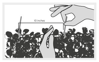
• To begin installing your greenery panels, place the first panel at the top of the metal fence and secure it with plastic zip ties. To prevent the panel from lifting, place additional plastic zip ties at an approximate distance of 10 inches.
