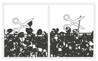
• Once the first panel is installed, connect the second panel, and secure it with plastic zip ties. Repeat the procedure until the entire work area is covered. • With scissors, trim any excess artificial greenery and the extra length of the plastic zip ties.
