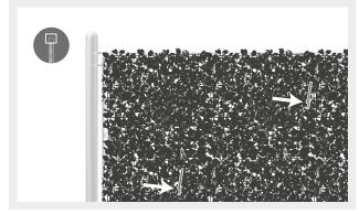
• Ensure the installation is secure by using additional plastic zip ties within artificial greenery. This will prevent the panel from coming loose.
