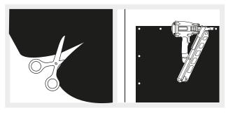
• Dark Fabric Installation: Cut the dark fabric to the size of the area you want to decorate. Use a manual stapler or nail gun to attach the fabric to the drywall. Start by installing the fabric in its corners and then inside, make sure to tightly stretch the fabric.
