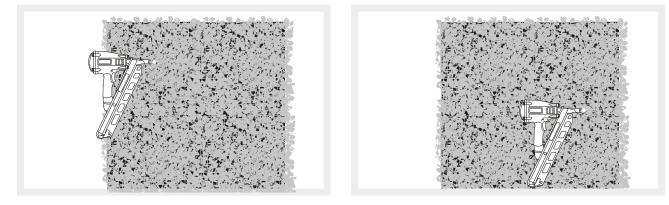
• Ensure the installation is secure by using additional staples within artificial greenery. This will prevent the panel from coming loose.
