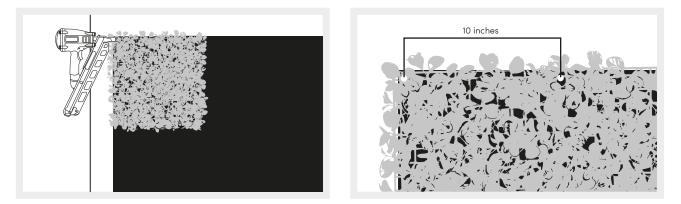
• To begin installing your greenery panels, place the first panel in the upper left corner and use a manual stapler or nail gun to secure it to the drywall. To prevent the panel from lifting, place additional staples at an approximate distance of 10 inches.
